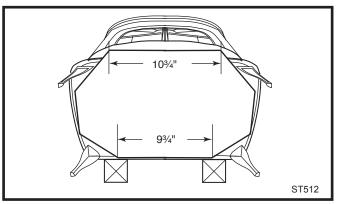
Fig. 14 Attach bottom heat shield.
